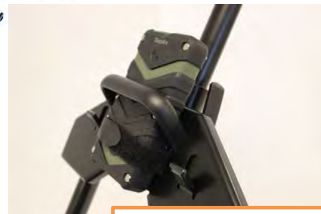
Battery Booster Installed
